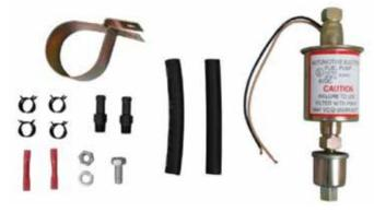
This pump can run on six or twelve volts. At six volts it puts out 25-30 GPH at 2.5-4.0 PSI, more than enough flow at an appropriate pressure for vintage vehicles. They are readily available at about \$35.00. I recently purchased two from Amazon.com. This style of pump works just fine in continuous operation as well.
