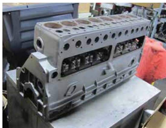
Figure 3: Cleaned and machined C11 engine ready for reassembly
