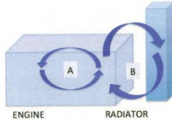
This leaves an insulating vapor in contact with the heat sources instead of the much more effective liquid coolant, and the resulting heat retention can cause damage.
