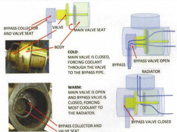
(horizontally in this view) as it is warmed by the coolant. In the center is the main body, and on the left side is a sliding valve assembly operated by the bellows.
