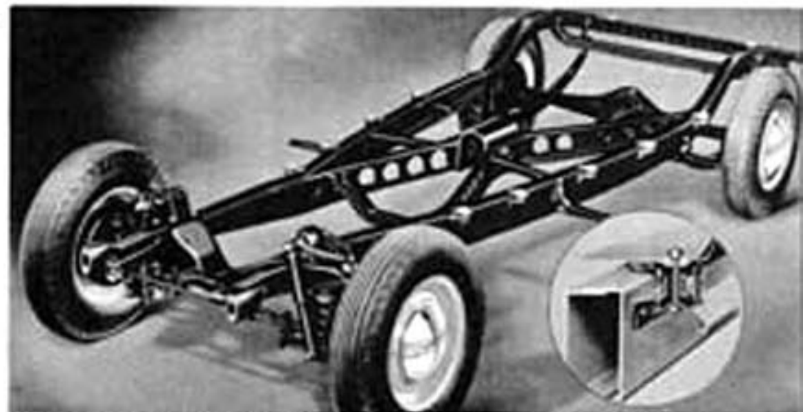
NEW OUTRIGGER BODY MOUNTINGS . . . although the Chrysler safety all-steel body follows the contour of the frame it no longer is mounted directly to it . . . it is mounted on short outriggers that are completely insulated with pure gum rubber . . . eliminating any metal to metal contact . . . noise can't be transmitted from frame to body.
