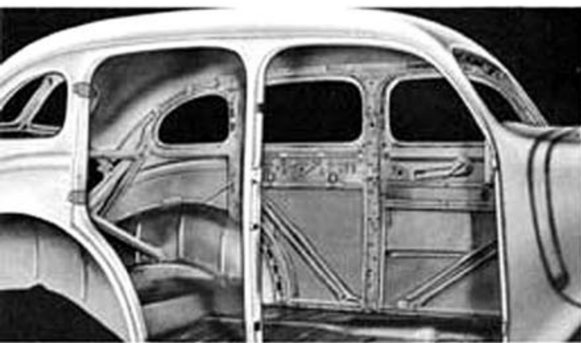
ALL STEEL BODIES . . . Chrysler safety all-steel bodies are built like a modern skyscraper—steel above, steel below, steel on all sides—all reinforced with steel, interlocking with the frame to provide the most rigid, safest bodies built. There are no bolted or screwed joints to cause leaks.
