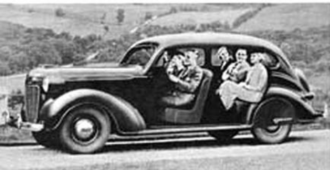
FLOATING RIDE . . . the engine and seats in the new Chrysler have been moved forward, so that weight masses have been redistributed and passengers ride between the axles where there is no jolting or bouncing as you glide over ordinary road irregularities.
