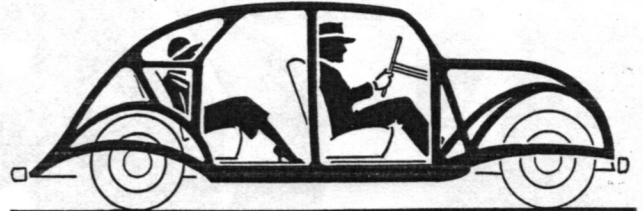
The Airflow De Soto is built like a steel bridge—with vertical and diagonal bracing throughout for maximum safety.
