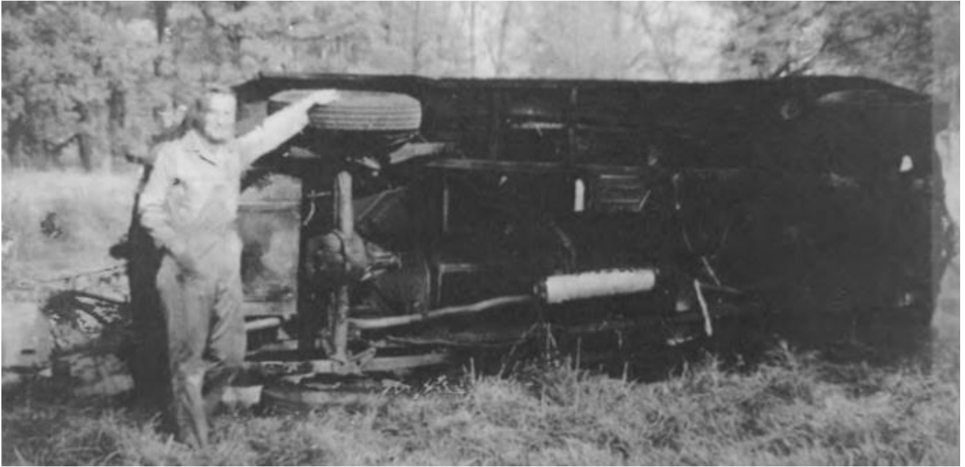
The only known photograph of any of the events that led up to and included the First Annual Airflow Demolition Derby. Nerf was leading the pack during the stock car race at Tribune when his front U-joint broke, the drive shaft dug into the dirt and flipped the C-10 off the track. Note missing drive shaft, and drive shaft retainer bracket. Nerf, who was unhurt, posed for the picture taken by a local newsman, shortly after Kramer's SE, Stewball II, won the event. Unfortunately despite thorough research no pictures of Kramer's '34 Desoto Coupe or of the City of Garden City have been unearthed to date. Photo courtesy of Garden City Daily Examiner, July 1952.
