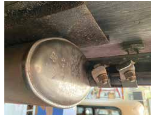
Figure 13 Rear muffler clamp and DeSoto-only heat shield
