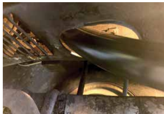
Figure 7 Head pipe clearance
