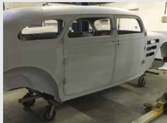
Sitting on the dolly, body finishing and paint can now begin.
