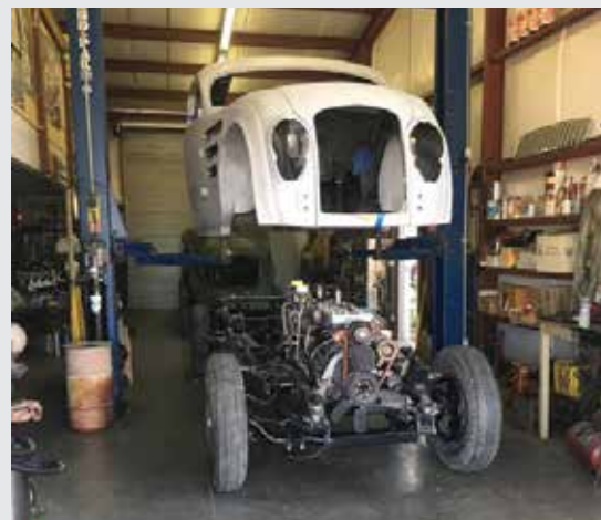
Body lift in progress. Plenty of headroom in the shop saves removing the wheels for this step.
