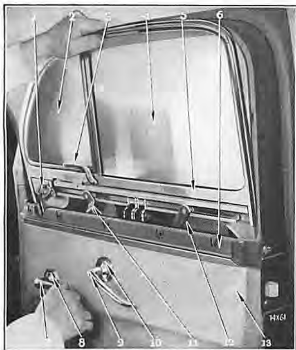
FIG. 16—Removal of Door Window Assembly
