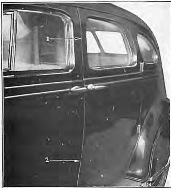
FIG. 9—Rear Door Sprung and Out of Alignment
