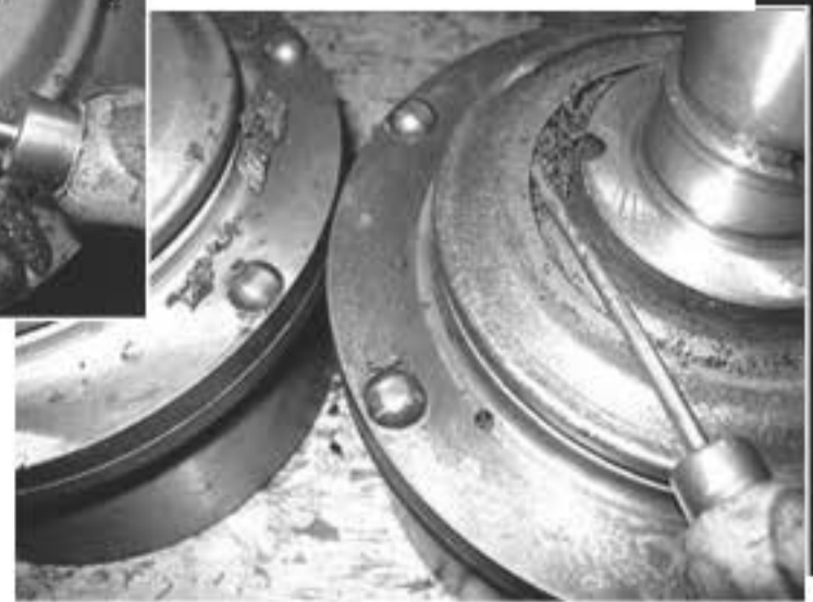
Disassembling and gouging out the hardened wax is the only way to get rid of this overdrive killer.
