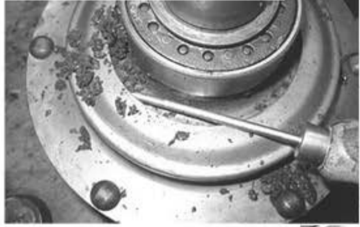
Above top: Three overdrive freewheel housings being cleaned out, middle: first of the three units getting cleaned; right: the second unit getting cleaned
