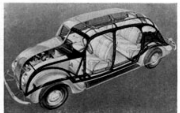
This is a model of De Soto's all-steel unit-frame-and-body. It is 40 times more rigid than the ordinary type. It means greater safety than ever before.
