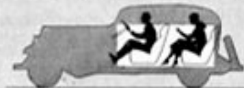
This diagram (above) shows how you ride in a conventional car. Pity the passengers riding over the back axle!
